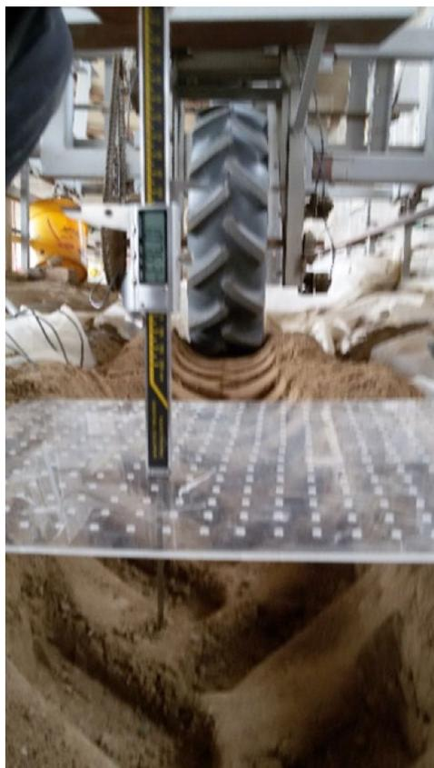
Figure 4. Measuring soil sinkage by means of a digital caliper and a Plexiglas plate.
