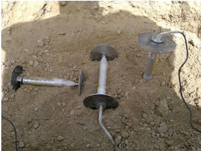
Figure 3. The arrangement of displacement transducers in three coordinate directions inside soil profile.
